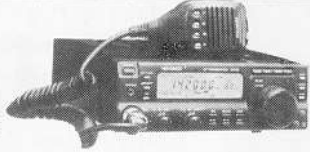
Kenwood TS 50 S HF-transceiver 160/10m, mode: AM, FM, SSB, CW.
